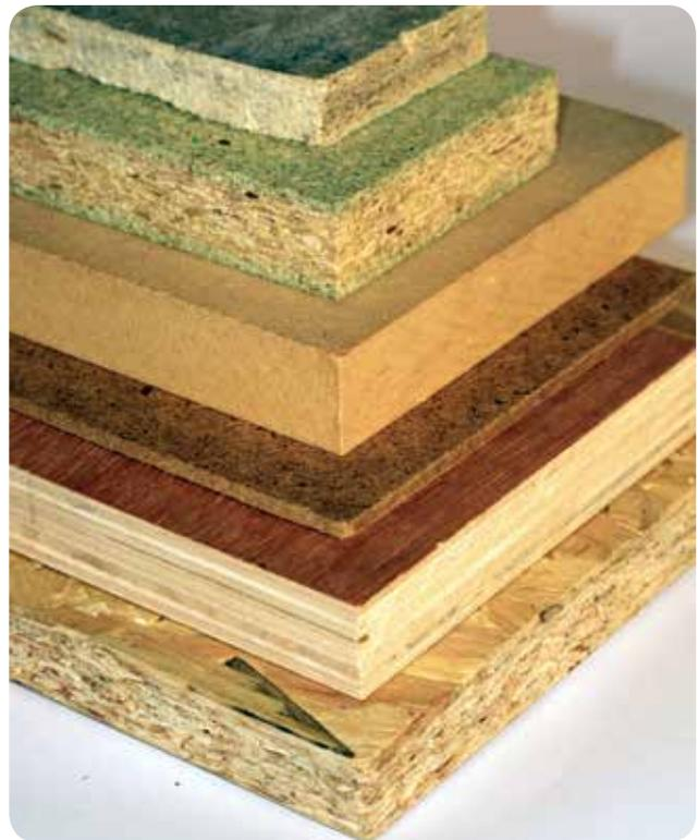
**Figure 1:** Wood-based panels, from top: cement bonded particleboard, chipboard, MDF, hardboard, plywood and OSB
