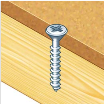
Screw for fixing thin attachments
