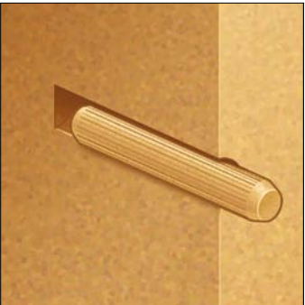
Dowel with 0.1mm all round clearance preferred
