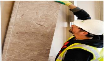
Pattress Plus is designed to provide support for fixtures and fittings in non-structural dry wall partitions. The product is an engineered OSB/3 panel incorporating a continuous recess, designed to accommodate 'C' shaped metal studs used in the construction of plaster board partitions.
