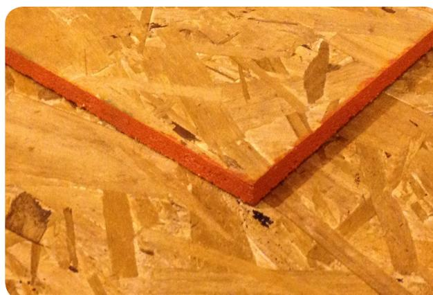
**Figure 1:** SmartPly oriented strand board, treated during manufacture.
