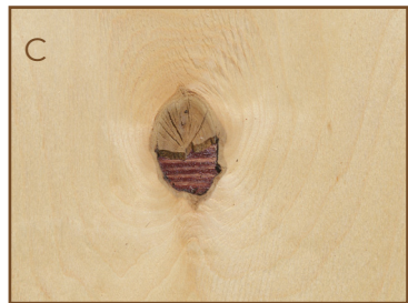
The lowest quality birch plywood. Usually unsanded and allows unlimited open defects.
